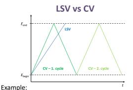
In the figure LSV measurement is carried out with the lower rate than CV measurement.
